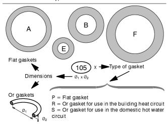
The dimensions of flat gaskets are indicated by the actual—size representation (A, B, C, D, E) in the figure above.
